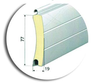
The 77mm standard lath requires at least 300mm (1ft) above your opening height to allow for the door to roll up into the box above. The lath is 77mm high and 19mm thick fully insulated.
