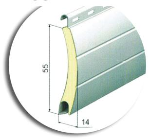
The 55mm lath requires at least 205mm above your opening height to allow for the door to roll up into the box above. The lath is 55mm high and 14mm thick fully insulated.
